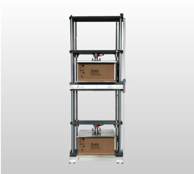
Figure 1: Stacked version of Kappa 10 DS with compression plates for creep test with corrugated cardboard boxes
